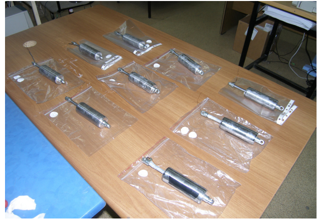
Fig. 6 Dampers after assembling
